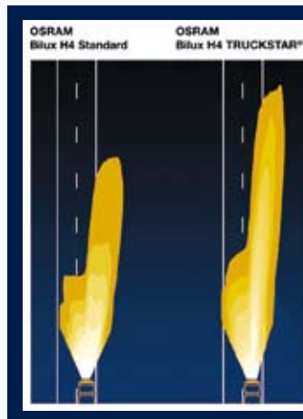
The OSRAM TRUCKSTAR® offers up to 100% more light on the road in comparison with a traditional 24V lamp (left)*.
